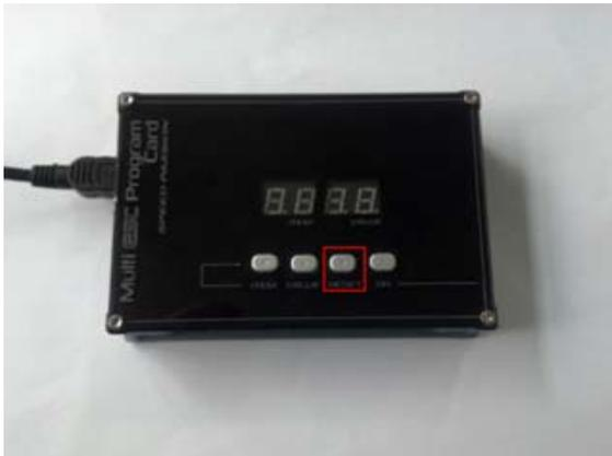
4. The program card will be display “- - - -”. Release the RESET button and launch the “Speed Passion Reventon PC Interface” program.
